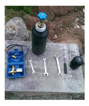
4. **Install a nitrogen gauge to measure the nitrogen pressure.** Screw the nitrogen gauge on the screw of the filling port according to the instructions, and then start to measure the nitrogen. But before measuring the nitrogen, make sure that the screw in the circle 2 is installed, if it is not installed, all nitrogen will be empty after test. Nitrogen measurement is to press the circle 1 to see how much gas left. After measuring, lift the needle on the circle 1 to get ready for the next step.
