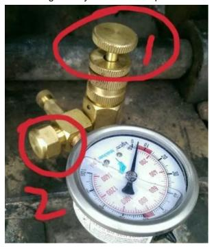
5. **Add nitrogen.** As shown in the figure, lift the needle at circle 1, and the nitrogen returns to zero. Then unscrew the screw at the circle 2, and connect the nitrogen gauge and the nitrogen cylinder with the air pipe.
