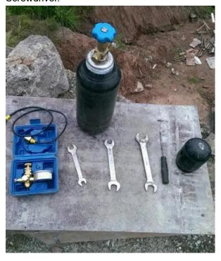
4. **Install a nitrogen gauge to measure the nitrogen pressure.** Screw the nitrogen gauge on the screw of the filling port according to the instructions, and then start to measure the nitrogen. But before measuring the nitrogen,
