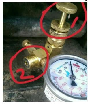
6. Now the wires have been connected and all the steps are ready. The last step is inflating. Please pay attention that the air filler valve in red circle as below picture must be lifted before inflating. Once turn on the blue plum blossom switch of the Nitrogen gas Cylinder, please depress the the air filler valve in red circle after the nitrogen
