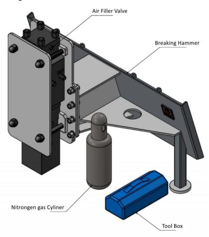
3. Please prepare Tool Box(included in the package), Nitrogen gas Cylinder(included in the package) and Screwdriver.
