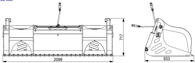
Inner Width 1220mm Universal Skid Steer Quick Attach:
