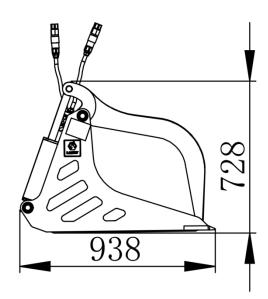
Inner Width 1220mm Universal Skid Steer Quick Attach:
