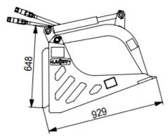
Inner Width 910mm Universal Skid Steer Quick Attach:
